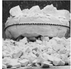
Fused Alumina ingots and lumps that are processed into micrometric sized powders
