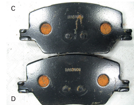
C Cu-free NAO formulation with conductive carbon black 2% TIMREX® T75 and 2% TIMREX® C-THERM™
