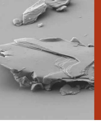
Mica is a naturally occurring, highly lamellar mineral. Micas are unique among platy minerals due to the transparent and luminous effect they impart. These optical effects are widely used in the cosmetics industry and are particularly in demand in make-up applications.
