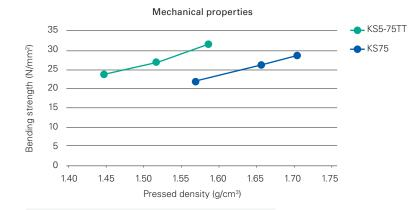
Dry mix (80/20) of graphite powder and phenolic resin. Pressed at 2,3,5t/cm<sup>2</sup>. Thermal treatment.
