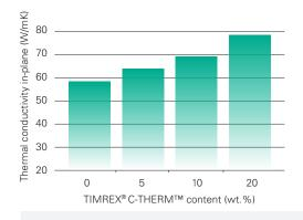
Dry mix (80/20) of carbon (TIMREX<sup>®</sup> KS150 + C-THERM<sup>™</sup>) and phenolic resin. Pressed at 2t/cm<sup>2</sup>. Thermal treatment.
