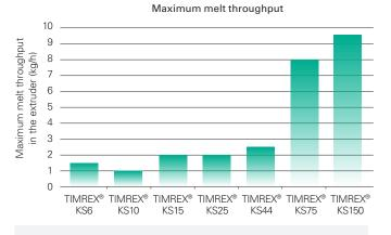
The production throughput of twin screw extruder and the energy costs can be improved by using coarse graphite d90 >75 microns.
