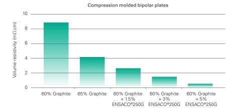
Polymer: Polypropylene Compound: Internal mixer Processing: Compression molding
