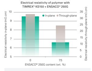
Dry mix (80/20) of carbon (TIMREX® KS150 + ENSCAO® 250G) and phenolic resin. Pressed at 2t/cm<sup>2</sup>. Thermal treatment.
