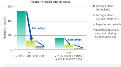
Polymer: Polypropylene (PP) Compound: Twin-screw extruder Processing: Injection molding
