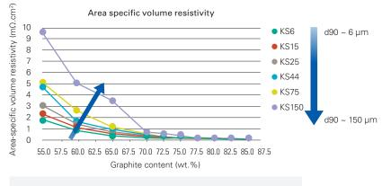
The percolation threshold is lower for fine graphite, but at higher graphite content the electrical conductivity is similar for all graphite particle sizes.
