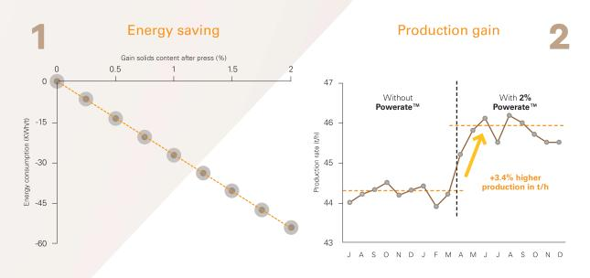
Each 1% higher dry content means savings of 96 MJ or 27 kWh per tonne board -27 Kwh/t for 44.2 t/h means saving of 1.7 M€ /y (KWh = 0.17 €)
